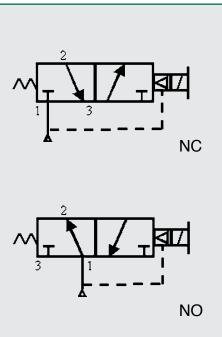
NOTE: 3-ported, 2 position valve (1/8" to 3/8") can be converted to a 2 way valve by inserting a pipe plug into the exhaust port.
