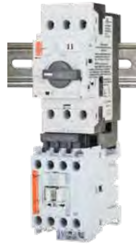
Remote Operation Application The KTU9 3-Pole unit can be combined with CA7 using Connector Modules to achieve remote operation. • For CA7-9...23 use KTU9-40H-PEC23
