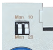
CEP7-1EE Switch Selection for Trip class (10 or 20)
